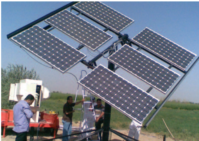
Setup of solar powered portable water filtration unit with solar tracking system and two stage RO and UF filtration process.
