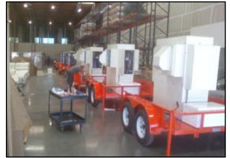
Solar powered, mobile, water purification units being manufactured at Mark's plant
